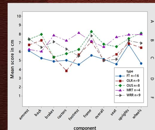
Figure 3. ANOVA interaction plot for wheelchair types: Folding transport chair (FT), Motivation Rough Terrain (M...), Whirlwind Roughrider (WRR); Other chairs made for low resource settings (OLR), and Other chairs made in the USA (OUS).
