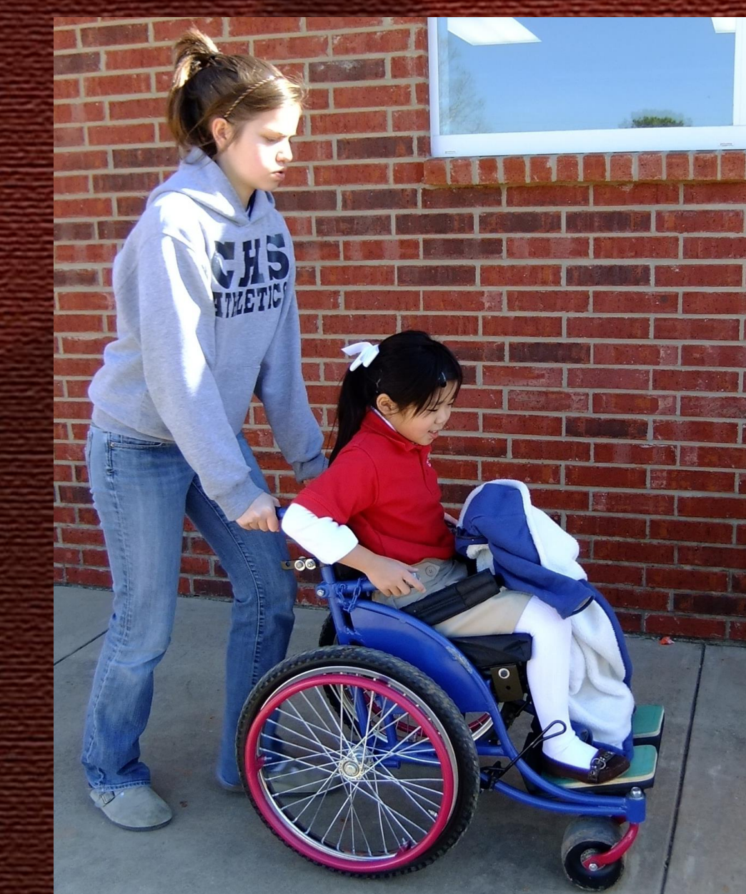
Figure 2. Subjects completing the energy cost assessment on smooth ground in the APDK 12" wheelchair
